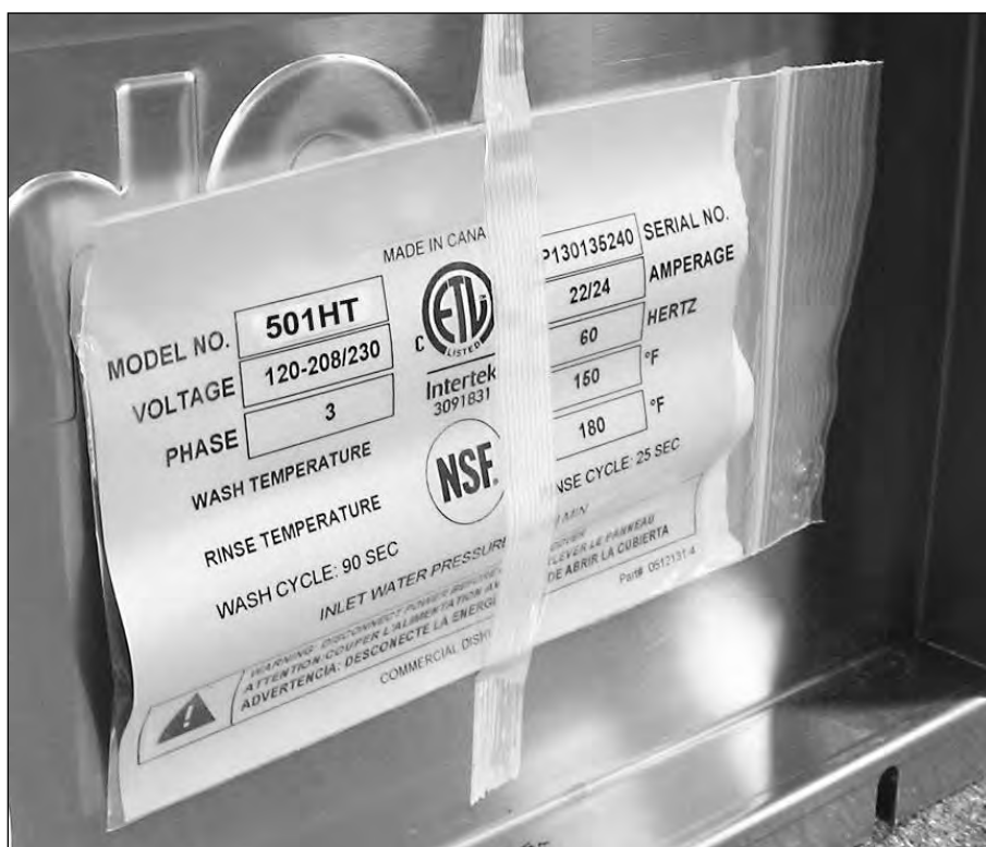
A three phase data plate is located on the back of the lower front panel.
