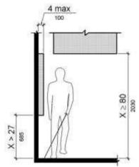
Figure 307.2 Limits of Protruding Objects Figure
