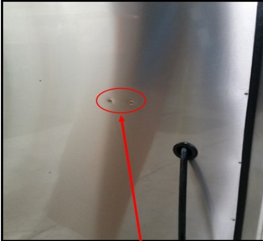
Step One: On Right Side, locate the two mounting studs.
