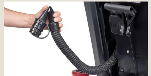
**Daily:** Empty the recovery tank using the recovery empty hose. Bend the soft part before removing the cap to control the flow.
