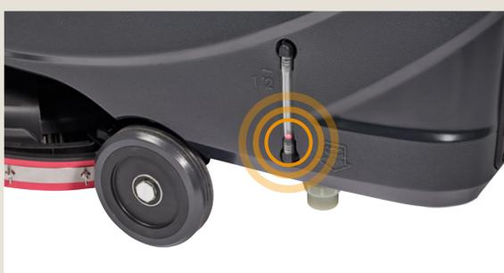
You can check the level of the solution anytime using the red ball on the left side of the machine.
