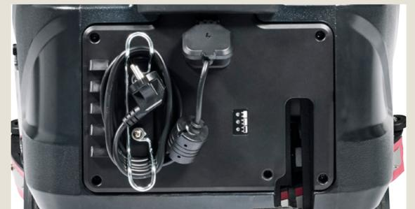
Charge the batteries whenever the machine is not in use. Connect the charger cable to the machine socket, then plug the cable into a grounded 3-prong electrical outlet. Red LED will be on during charging, and the Green LED will turn on when charging is complete.
