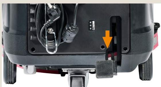
Lift the deck by pressing the pedal down and to the left. The squeegee is raised and lowered with the deck.
