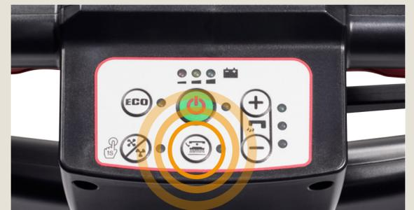
**Daily:** With the machine turned on and the deck lifted, press the click off button to release the brush/pad holder then clean and inspect before next use.
