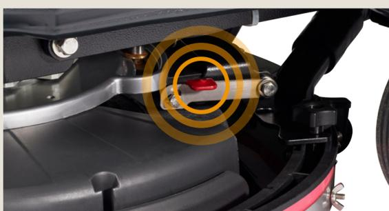
Lift the squeegee up by hand until it locks in the UP position, and turn off the vacuum, to perform double scrubbing. To return to normal working mode, use the red lever to release the squeegee, and turn the vacuum back on.
