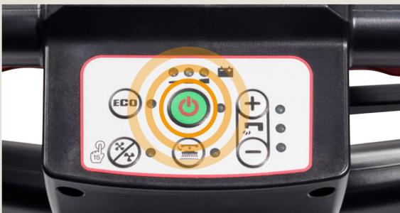
When scrubbing is complete, turn off the on/off button to perform the following maintenance.
