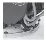
For a full functioning scrubber, move the hose to the squeegee and lower the squeegee to the floor.
