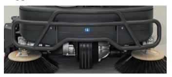
Don't let the smooth, precise acceleration of its maintenance-free AC brushless propulsion drive fool you. With an industrial bumper, frame-mounted deflectors and a tubular, steel construction all specifically engineered for the most severe industrial applications, the SC6500 is as tough as they come and built to last.
