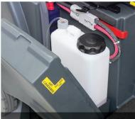
Removable, high capacity detergent cartridge for sustained flexible cleaning is available with optional EcoFlex™ System.
