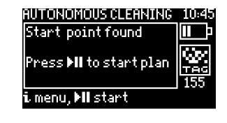
Drive to the start point of an existing plan. The above screen should appear.
