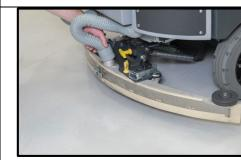
Make sure squeegee is clean and ready for use. Connect the recovery hose to the squeegee inlet using hose clamp.
