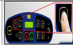
Press the solution switch once to turn off solution flow while making sharp turns.
