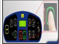
Press the green Scrub On Switch to activate the scrub system. Set the chemical dilution ratio. Begin scrubbing.
