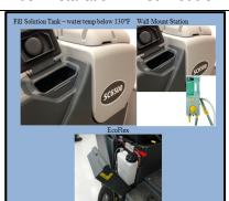
Fill machine with water (add detergent as required). Fill solution tank with water only if using EcoFlex (refer to owner's manual).
