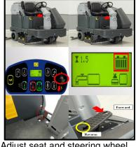
Adjust seat and steering wheel. Turn machine on, verify battery power, release brake, and drive to fill station.
