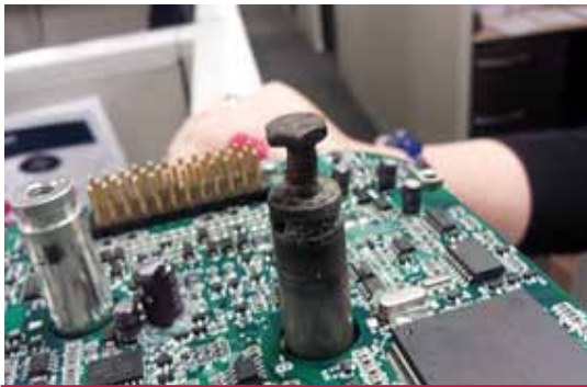
Figure 14: Damaged Controller lug from loose connection. (Case removed for clarity)
