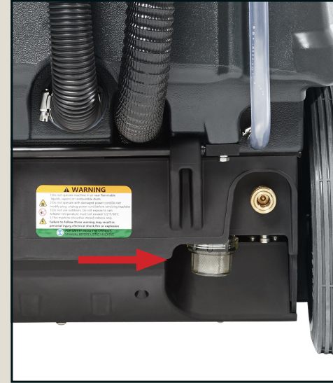
At the bottom of the machine you can access to the solution filter. Keep the filter clean
