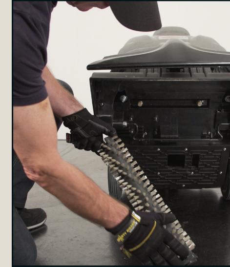
Pull the brush out by the left side and clean it. To install again connect the right side first then push the left side of the brush in place. Remove the suction nozzle and clean it
