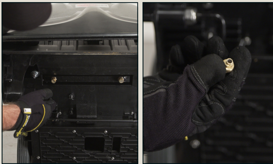
When the brush is removed clean the brush housing and if needed check the two spray nozzles
