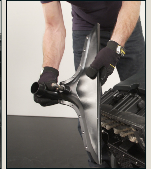
Pull the brush out by the left side and clean it. To install again connect the right side first then push the left side of the brush in place. Remove the suction nozzle and clean it
