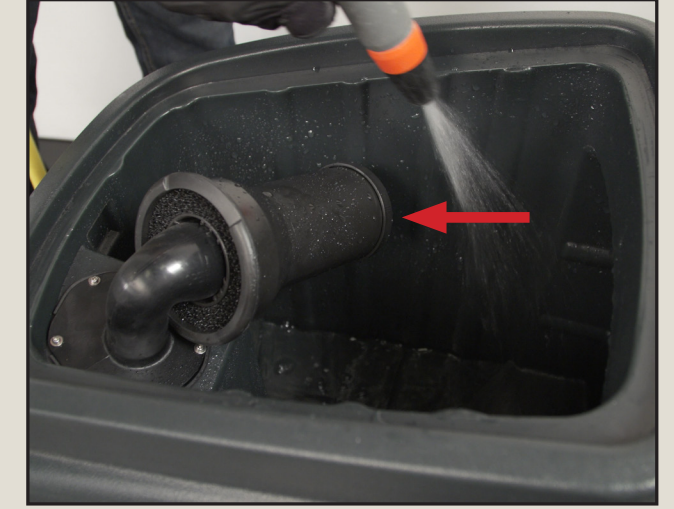
Clean the float ball system inside. Clean the lid gasket
