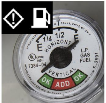
Check the Diesel fuel tank level / LPG bottle charge. In case re-fill/ change the LPG Bottle
