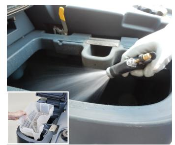
14. Wash with clean water the recovery tank and the vacuum grid. Remove and clean the debris tray.
