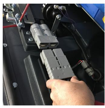
**2** For the battery version check the battery voltage and if needed recharge
