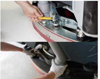
2. Check the fresh water level. In case, 3. Fill the EcoFlex™ tank (placed under 4. Install the squeegee and fasten it to its assembly then connect the vacuum hose to the squeegee. Make proper height and inclination adjustments
