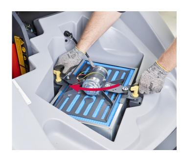
16. Dump the hopper, remove and clean the filter
