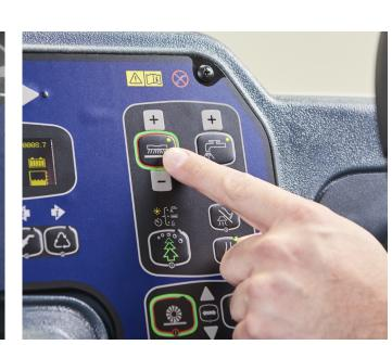
8. Press One-Touch™ scrub (adjusting the pressure if needed) and One-Touch™ sweep buttons according to your application
