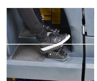
11. Press the forward pedal and start operating the machine
