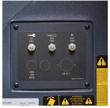
**4** Inspect the circuit breakers
