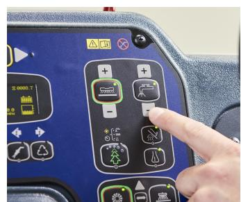
9. Adjust to the desired water flow
