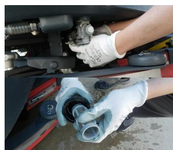
15. Close the solution tank valve and remove and clean the filter. Ensure sealing gasket remains in filter cap
