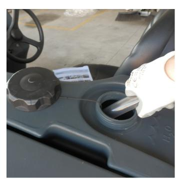
**1** Enough water in the solution tank? **2** Solution valve open?
