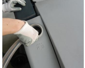
6. Fill in the DustGuard™ water tank (if equipped)
