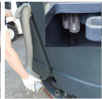
**4** Squeegee hose free from debris. Verify recovery tank is not full and float balls are blocking motor inlet
