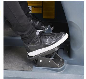
**3** Drive pedal must be released during engine cranking
