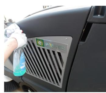
20. Clean the machine using a damp cloth and park it with the recovery tank open
