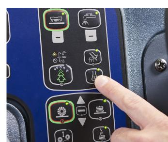
10. Adjust to the desired chemical concentration (shown in the display)
