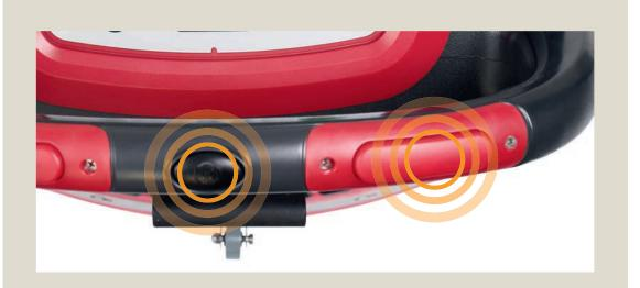
Pressing either of the red safety switches and the black reverse button together will put the machine into reverse.
