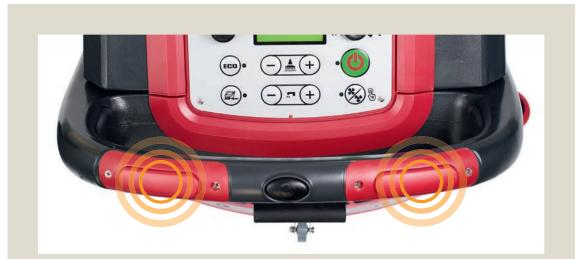
Press the One button start icon and then press and hold any of the two red safety switches to activate the machine.
