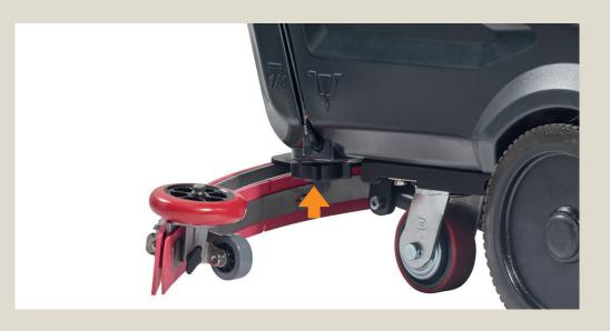
**Daily:** Place the rear of the scrubber over a floor drain. Empty the clean water tank using the solution tank drain knob under the machine.
