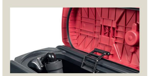
**Daily:** Leave the recovery tank lid open after it's been cleaned to air out and avoid any odor formulation.
