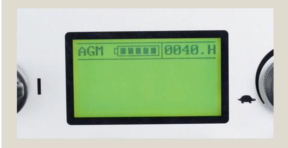
**Daily:** Charge the machine at the end of the cleaning shift or if the battery indicator is low or showing empty.
