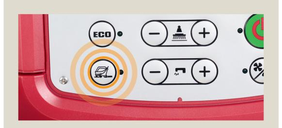
Press the Floor Finish Removal icon (orbital only) for removing finish: pad pressure will be set to maximum, solution flow will be set to minimum & machine speed will be held at 1.0 km/h (0.6 mph).
