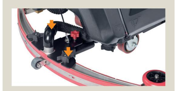
Install the squeegee using the thumb nuts. Attach squeegee hose.
