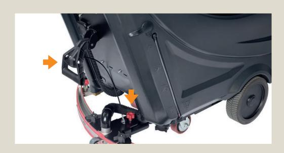
Use the handle to lower or raise the squeegee to the floor. Adjust the squeegee angle with the knob to maximize solution pickup performance if necessary.
